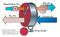
In the 1950's Munters invented modern industrial dehumidification when it introduced the selfregenerating desiccant rotor, the heart of the dehumidifier.
